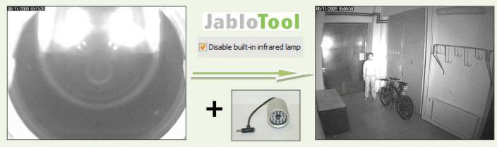
Using an external PIR and IR lamp
